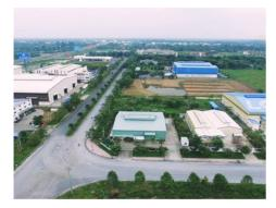
Transportation system The main road is 45m wide, the internal road is 24-35m wide, covered with hot asphalt concrete and designed to withstand a load of H30 according to Vietnamese standards.
